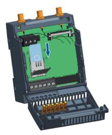
4. Lock the card holder in the marked direction.
