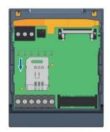
3. Put the SIM card in the card holder and then lock the card holder in the marked direction.
