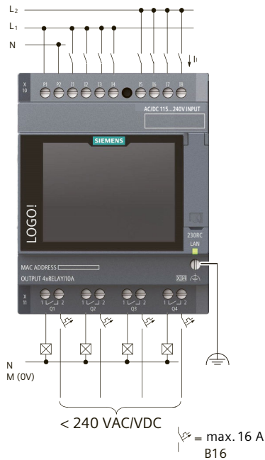
Two-phase connection of the Base Module
